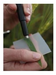
1. Place the leaf cutting mat under the leaf to be sampled. There is no requirement to remove the whole leaf from the plant.
