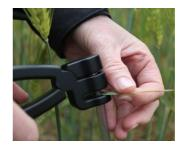
2. Slide your leaf between the top of the tube and the edge of the round cutting blade. Squeeze the handles of the tool together to punch a leaf disc into the 2D-barcoded tube.
