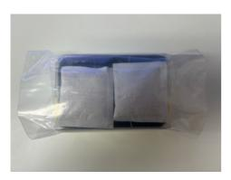
5. Expel as much air from the bag as possible and then close the seal. This step seals in the remaining air around the samples and allows the desiccant sachets to absorb moisture from the sample to reduce the chance of fungal growth.
