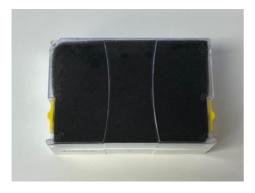
2. Once the rack is filled with your sealed sample tubes, place the sponge pad on top of the tubes, and securely close and lock the lid of the rack.
