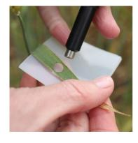
2. Press the leaf cutting tool into the leaf and onto the leaf cutting mat. Twist the tool through the leaf and onto the mat as it cuts. The cut leaf disc leaf will remain in the tool.
