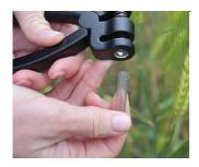
1. Select an empty 2D-barcoded tube from the rack provided and remove the lid. Insert it into the base of the advanced leaf cutting tool.
